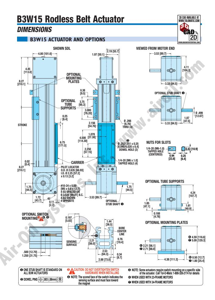
Unless otherwise noted, all dimensions shown are in inches [Dimensions in brackets are in millimeters]
