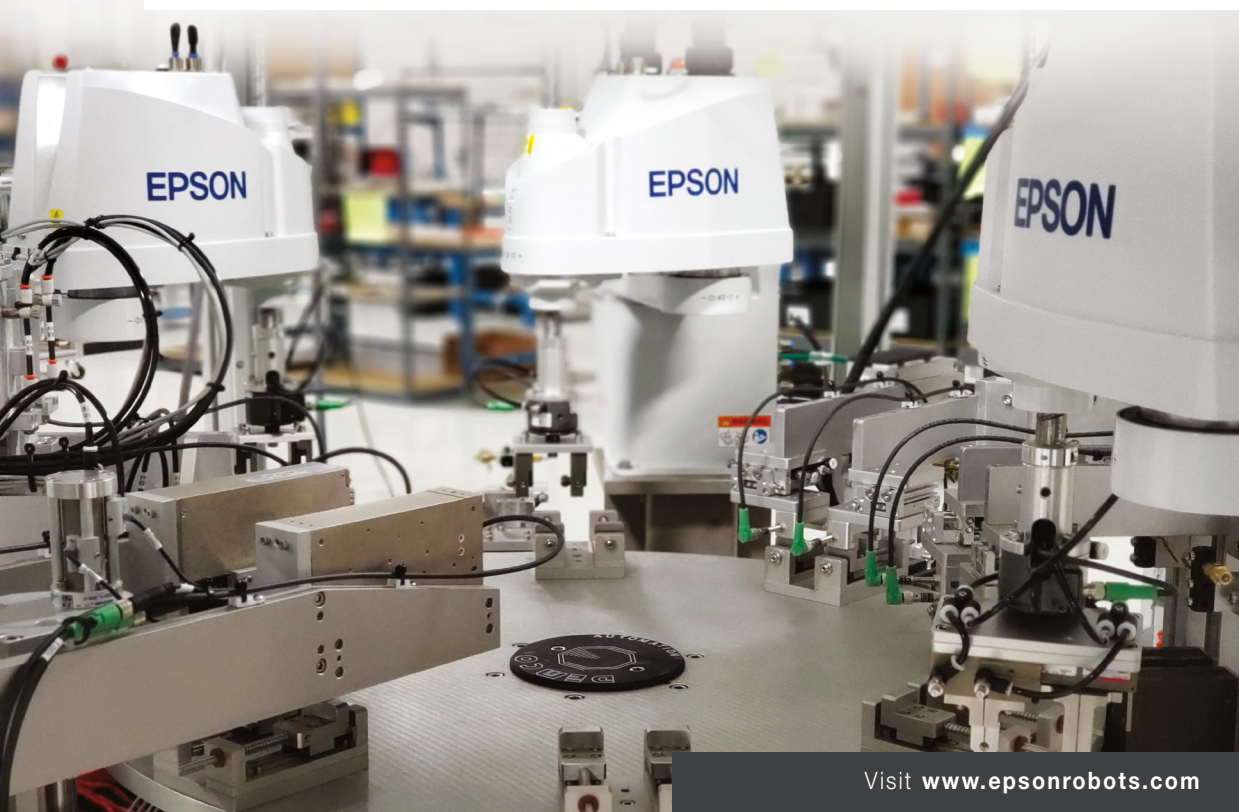
Multi-robot assembly system with (3) Epson T3 SCARA Robots for surgical instrument forming and packaging system. Courtesy of Demco Automation
