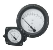
NOSHOK 1000 SERIES PISTON TYPE DIFFERENTIAL GAUGES are designed for measuring pressure drop across filters, strainers, separators and valves. The single piece construction of the ceramic magnet/piston is designed to reduce "blow by" and increase gauge accuracy. These gauges can be found in applications requiring high differential pressure from 0 to 5 psid to 0 to 100 psid with maximum working/static pressure to 6000 psig.
