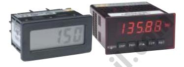
NOSHOK 1000 SERIES HIGH PERFORMANCE DIGITAL PRESSURE GAUGES are designed to exceed the industry's most demanding application requirements. Using the latest in reliable ceramic thick film strain gage technology combined with low power electronics, these gauges are accurate, stable and extremely reliable. The 1000 SERIES gauges are ideally suited for local indication and with the analog voltage output or limit switch option they can interface with other monitoring and control systems.
