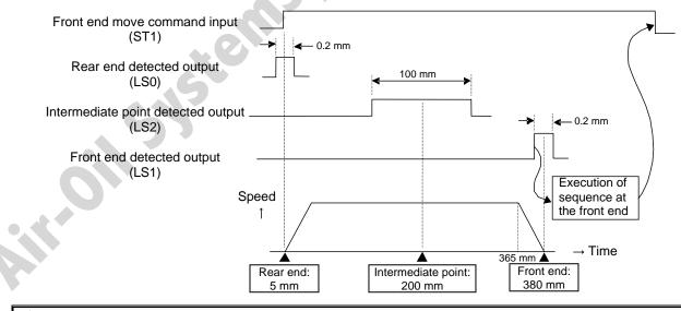
/ Caution: Provide a ladder sequence circuit where only one move command signal turns ON at a time. If two or more signals are input at the same time, the signals will be processed in the following priorities: Priorities: [1] Rear end, [2] Front end, [3] Intermediate point
