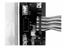
Connect the supplied flat cable. Connect the opposite end of the cable (no connector) to an appropriate peripheral (host PLC, etc.).
