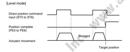
(Note) Turn OFF the movement command input after confirming that the target position has been reached.
