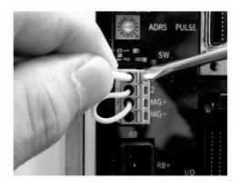
As shown to the left, insert the stripped end of the cable while pressing down the spring using a screwdriver. Applicable cable diameter: 0.2 to 1.3 mm (AWG24 to 16) Recommended stripped wire length: 10 mm
