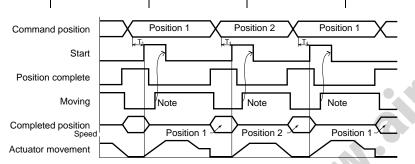
T1: 6 msec or more; time after selecting/entering a command position until the start input turns ON (The scan time of the host controller must be considered.)
