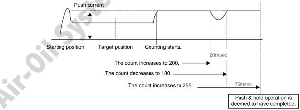
If the motor current remains at or above the push current for 200 msec and then drops below this level for 20 msec, the count will decrease by 20. When the push current is reached again thereafter, counting will start from 180. If the motor current remains at or above the push current for 75 msec, the count will increase to 255 and thus push & hold operation will be deemed to have completed. In total, 295 msec was required for the judgment.
