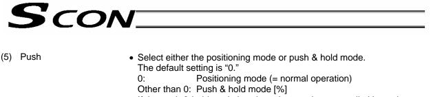
If the push & hold mode is selected, enter the current-limiting value to be applied to limit the AC servo motor current during push & hold operation.
