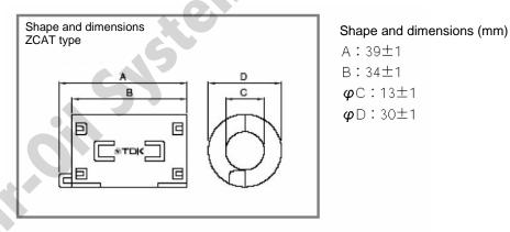
[Fig. 2] External View of Clamp Filter
