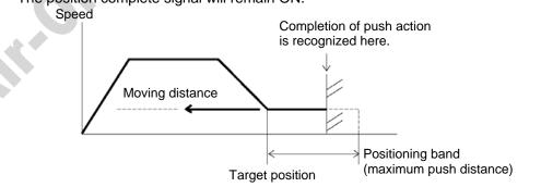
(Note) If the actuator is pushed back to the target position, an "out of push & hold operation range" alarm will generate.
