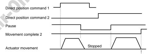
The target position is where movement complete 2 turns ON.
