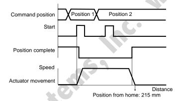
If the start signal for movement to an incremental position number is input multiple times during positioning, the actuator will move to the position corresponding to the initial position plus the "increment x number of times the signal was input."
