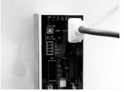
Use the pulse-train control cable when the controller is operated in the pulse-train input mode. It should not be connected when the controller is operated in the positioner mode.
