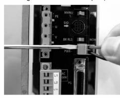
As shown to the left, insert the stripped end of the cable into the connector and screw in the cable using a screwdriver. Applicable cable: 0.75 to 1.25 mm Recommended stripped wire length: 7 mm
