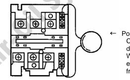
Point Connect to each coil over the shortest possible wiring distance.
