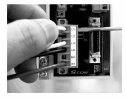
As shown to the left, insert the stripped end of the cable into the connector and screw in the cable using a screwdriver. Recommended cable diameter Motor power (L1, L2): 2 mm (AWG14) Control power (L1C, L2C): 0.75 mm (AWG18) Recommended stripped wire length: 7 mm
