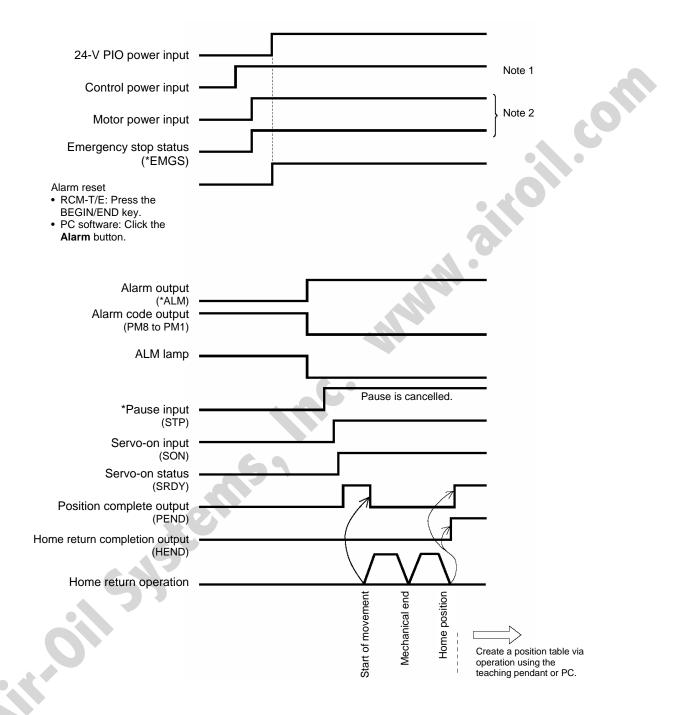
Note 1) Always input the 24-V PIO power (and the 24-V brake power if the actuator is equipped with a brake) before the control power and motor power.
