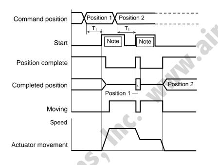
T1: 6 msec or more; time after selecting/entering a command position until the start input turns ON (The scan time of the host controller must be considered.)
