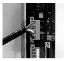
Connect the motor cable of the actuator to the motor connector on the front face of the controller.
