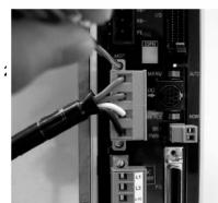
Use a screwdriver to tighten the screws at the top and bottom of the connector to secure the connector.
