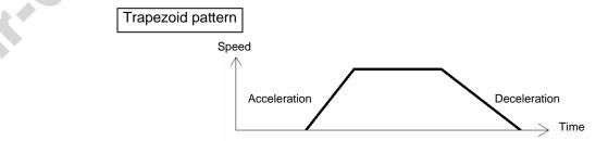
\* Set desired acceleration and deceleration in the "Acceleration" and "Deceleration" fields of the position table.
