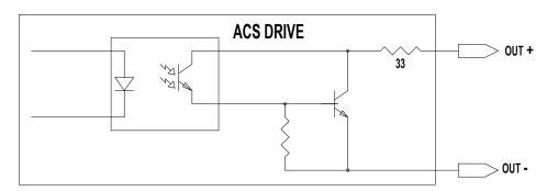
Figure 6-6: Output Circuit
