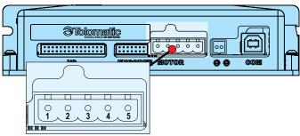
Figure 5-1: Motor Power Connection on ACS Drive
