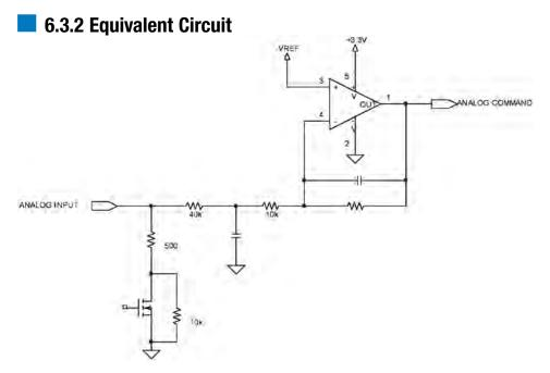
Figure 6-9: Analog Input Equivalent Circuit
