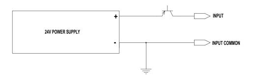
Figure 6-3: Input Source (PNP) Connection
