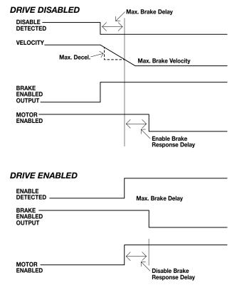
Figure 7-5 Brake Subsystem Timing
