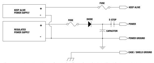
Figure 6-16: Regulated Power Supply Configuration with Blocking Diode and Added Capacitance
