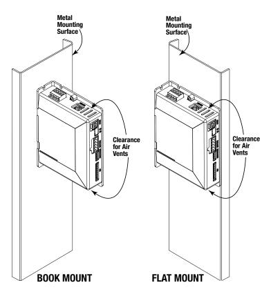
Figure 2-2 Mounting the ACS Drive
