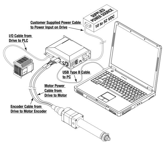
Figure 4-1: ACS Drive and ERD Actuator – Basic Setup
