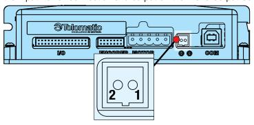
Figure 5-8: Brake Connection
