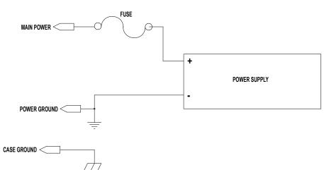
Figure 6-13: ACS Drive Single Supply - Main Power
