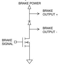
Figure 6-11: Brake Output Equivalent Circuit
