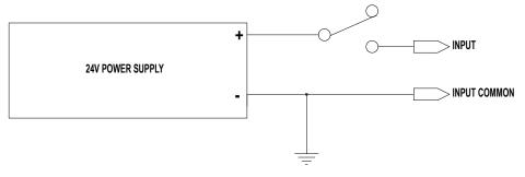
Figure 6-2: Input Source (switched) Connection
