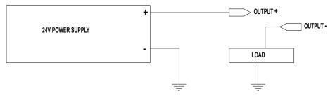
Figure 6-8: Digital Output Sourcing Connection
