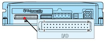
Figure 5-5: I/O Connection on ACS Drive
