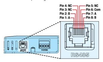
Figure 5-11: ACS 2-Wire RS485 with RJ45 Socket
