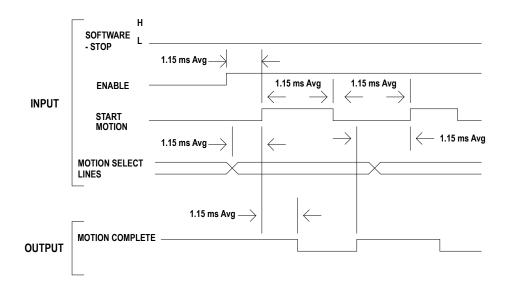
Figure 7-4 Absolute & Incremental Move Timing
