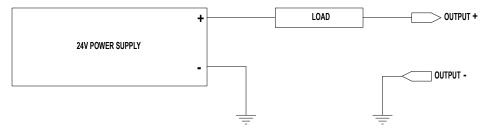
Figure 6-7: Digital Output Sinking Connection
