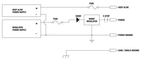
Figure 6-17: Regulated Power Supply with Blocking Diode and Shunt Regulator
