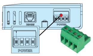
Figure 5-7: Input Power Connection
