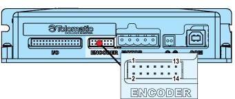
Figure 5-3: Encoder Connection on ACS Drive
