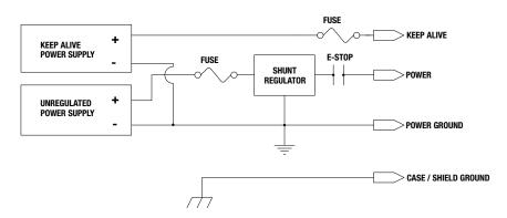
Figure 6-15: Unregulated Power Supply Configuration with Shunt Regulator
