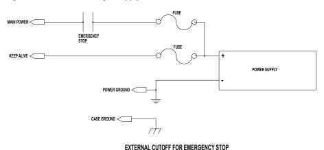
Figure 6-14: ACS Drive External Cutoff Switch for Emergency Stop
