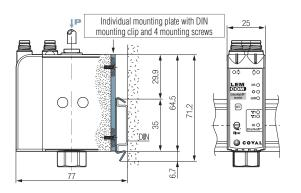
For static mounting (for example, in a cabinet), a module can be clipped onto a DIN rail. For this purpose, the module must first be equipped with an individual plate for mounting onto a DIN rail
