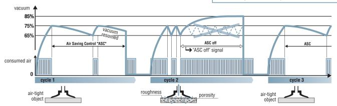
Specially designed by COVAL, the **LEMAX+** vacuum pumps integrate the **ASR** (regulator-venturi) combination which greatly reduces the compressed air consumption and noise level. See page 8/3.
