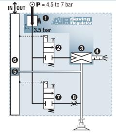
Combined "venturi regulator" **ASR**: pressure regulator **1** feeds venturi **2** with 3.5 bar, optimal for its operation.
