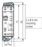
To mount from front, in addition to the module, a mounting kit must be ordered:
