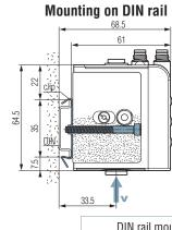
DIN rail mounting kit: 2 clips + 2 screws
