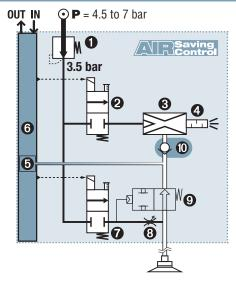
Combination of non-return @ and advanced electronics 6 ensures the ASC's automatic management.
