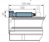
Mounting of the **VA** vacuum switch option for a gripper with vacuum generator (version **E1**, **E2** or **E3**) and not having sufficient space for the horizontal mounting.
