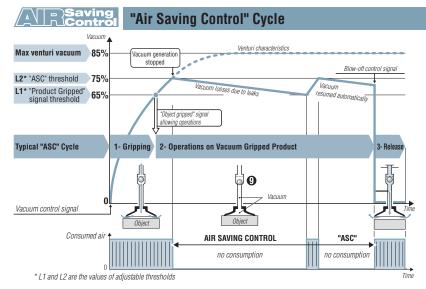
As illustrated above, the **LEMAX** module automatically executes the "**ASC**", cycle, thus saving the maximum amount of energy, based on the following 3 phases.
