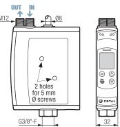
Mounting from side is the simplest to implement: Two  $\emptyset$  5 mm through screws or bolts with large washers.
