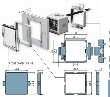
Panel opening (max. thickness: 4.5 mm)
