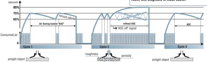
LEMCOM series vacuum pumps, which integrate an **ASR** "venturi regulator" combination, maintain ideals that COVAL values greatly: reducing both compressed air consumption and noise generation. See p. 8/28.
