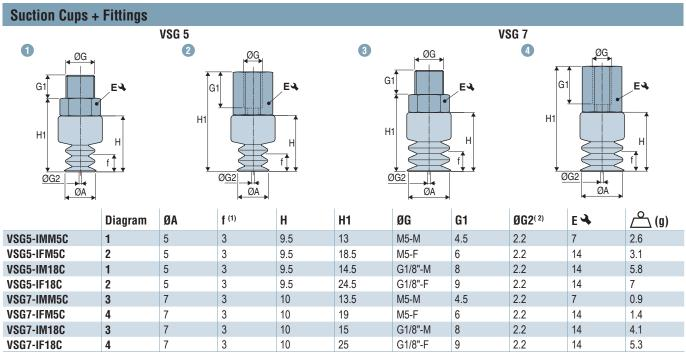
(1) f = Deflection of the suction cup. (2)  $\emptyset$  G2 =  $\emptyset$  internal orifice of the fitting.
