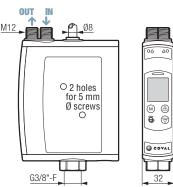
Mounting from side is the simplest to implement: Two  $\emptyset$  5 mm through screws or bolts with large washers.
