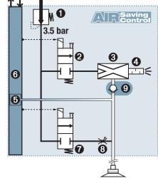
Combination of non-return **9** and advanced electronics **6** ensures the **ASC's** automatic performance.
