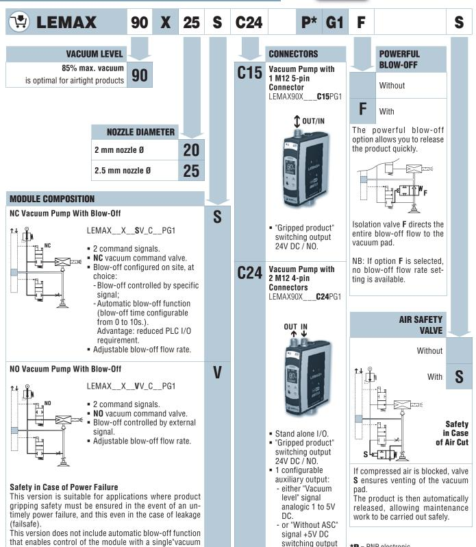
**EXAMPLE OF COMPLETE PART NUMBER: LEMAX90X25SC24PG1 LEMAX+** vacuum pump, 85% maximum vacuum, 2.5 mm nozzle Ø, controlled by a NC (Normally Closed) solenoid valve, connection by 2 M12 4-pin connectors.
