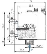
DIN rail mounting kit: 2 clips + 2 screws
