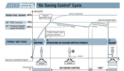
As illustrated in the above figure, the LEMAX module automatically executes the "ASC", cycle, thus saving the maximum amount of energy, based on the following 3 phases.
