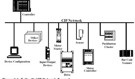
Figure 1.1: EntherNet/IP Network Example
