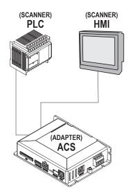
Figure 1-2: ACS Drive as an Adapter Device.
