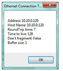
Figure 3-3: Testing Verifies a Successful Ethernet Connection
